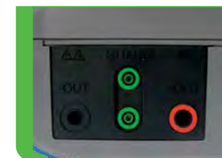
Guard terminal for connecting shielded test leads
