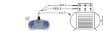
Test circuit for continuous resistance measurement
