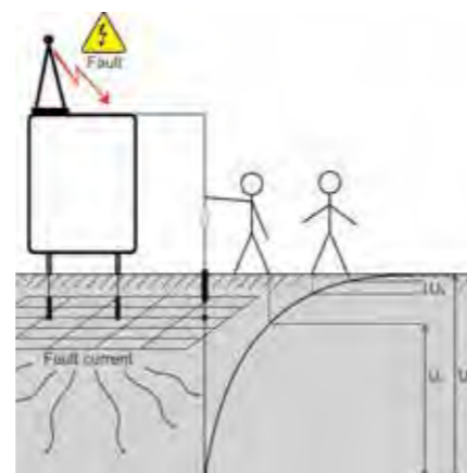
Dangerous voltages on a faulty earthing system
