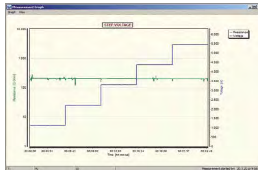
R(t) graph can be drawn for HV Insulation Resistance measuring functions.
