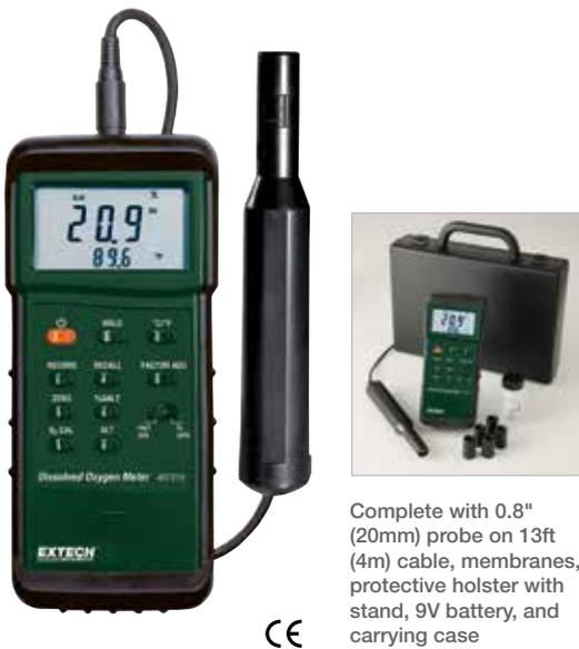
Complete with 0.8" (20mm) probe on 13ft (4m) cable, membranes, protective holster with stand, 9V battery, and carrying case
