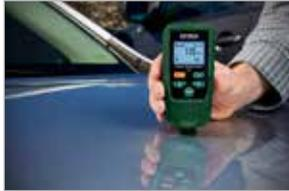
**Automatic recognition for ferrous and non-ferrous substrates with 1500 data storage and USB interface for further data analysis on a PC**
