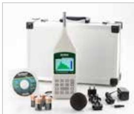
Includes Windows® compatible software, USB cable, 4 x C batteries, microphone wind screen, mini screwdriver, 120V AC adaptor, and case. See p. 122 for 220-240V Adaptor; 1yr warranty; Optional 94/114dB calibrator (see 407766 on p. 120)
