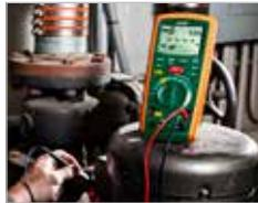
Insulation test on pump motor
