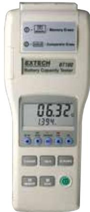
**AC milliohmmeter checks Battery Condition in seconds while the battery is in service**
