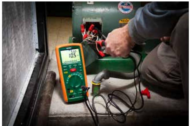
Insulation test on pump motor
