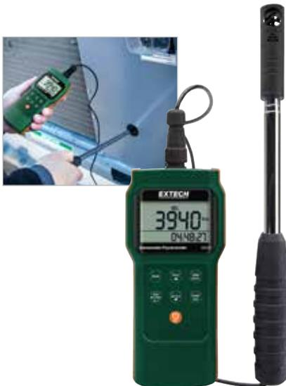
**Telescoping probe with 18mm diameter mini vane sensor easily fits into air vents and can extend length of probe to 3.3ft (1m) long**
