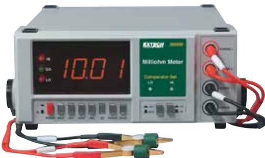
**Benchtop meter provides resolution down to 0.01mΩ**
