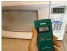
**Designed to measure high frequency radiation levels emitted from household and commercial microwave ovens**
