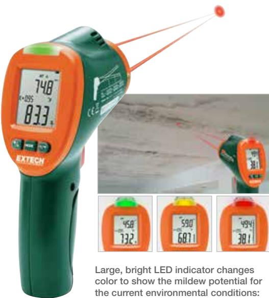
Large, bright LED indicator changes color to show the mildew potential for the current environmental conditions: Green LED indicates a very low potential; Yellow LED indicates a moderate potential; Red LED indicates a high probability for mildew formation
