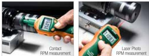
Contact RPM measurement
