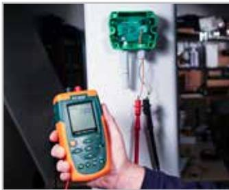
**“Source” for calibrating process devices and measuring DC process signals**
